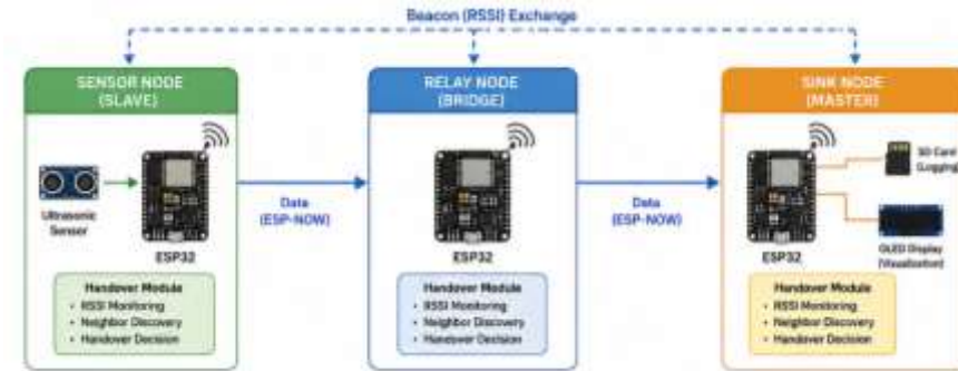
Fig.1 ESP-NOW Peer-to-Peer (P2P) Multi-Node Network with Handover Mechanism
